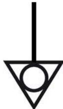
The equipotential conductor must have a minimum section of 10 mm<sup>2</sup>.
