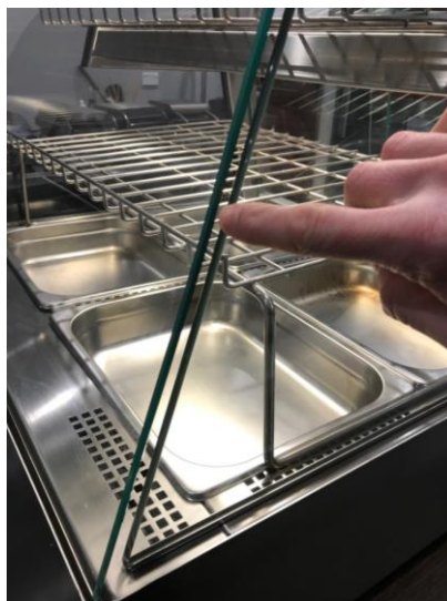
(Image shows glass gap for airflow)
